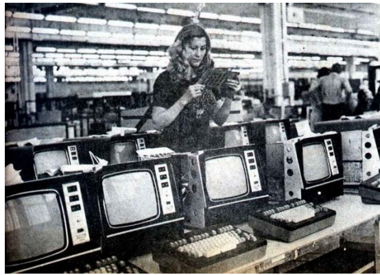
Assembly of the VIDEOTON VT 340 (EC-7168) graphical display terminals at VIDEOTON's Factory of Computer Technologies
