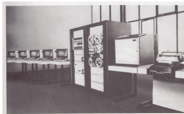
The Hungarian Ryad computer, the VIDEOTON R10 (EC-1010) with its VT 340 (EC-7168) graphical display terminals
