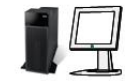
9114-275 (demo), IntelliStation Z75 workstation: - 2 way POWER4+ 1.45GHz, - 8 Gb memory, - POWER GXT6500 Graph.adapt.
