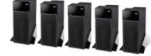
p650 + D20 exp drw: - 8way POWER4+ 1.45GHz, - 32 Gb memory, 5 x FC adap., - 4 x 10/100/1000 Eth., - LPAR, HACMP ready.
